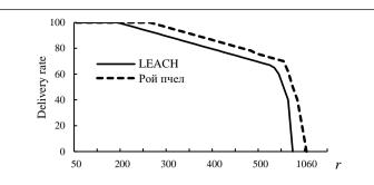
Fig. 2. The dependence of the value of the data packet delivery coefficient on the WSN operation duration
